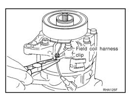
6. Remove snap ring using external snap ring pliers.
