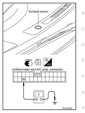
• When checking sunload sensor, select a place where sunshine directly on it.
