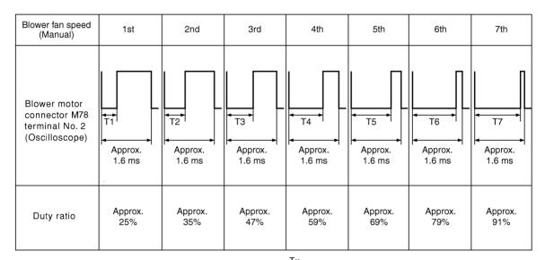
NOTE: Duty ratio =  $\frac{Tx}{Approx. 1.6 \text{ ms}} \times 100 \text{ (%)}$
