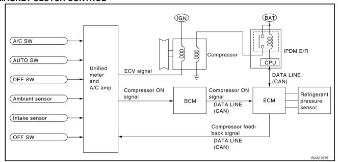
When A/C switch, AUTO switch or DEF switch is pressed, unified meter and A/C amp. transmits compressor ON signal to BCM.
