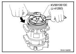
Remove clutch disc using a clutch disc puller (SST).
