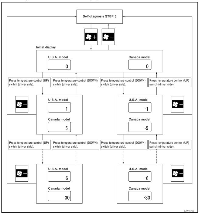
When battery cable is disconnected or battery voltage is below 10 V, trimmer operation is canceled. Temperature set becomes that of initial condition, i.e.  $0^{\circ}$ C  $(0^{\circ}$ F).
