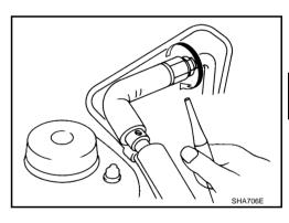
3. Move probe along component approximately 25 to 50 mm (1 to 2 in)/sec.
