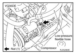
6. Remove mounting nut, and then remove low-pressure pipe (VK45DE).
