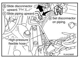
5. Remove mounting nut from high-pressure flexible hose (compressor side), and then remove high-pressure flexible hose.
