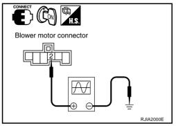
3. Change the fan speed from Lo to Hi, and check the duty ratios between blower motor harness connector M78 terminal 2 and ground using an oscilloscope. Normal terminal 2 drive signal duty ratios are shown in the table below.
