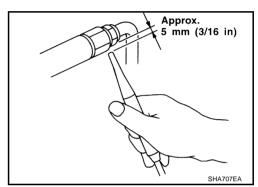
When testing, circle each fitting completely with probe.
