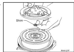
5. Using holder to prevent clutch disc rotation.
